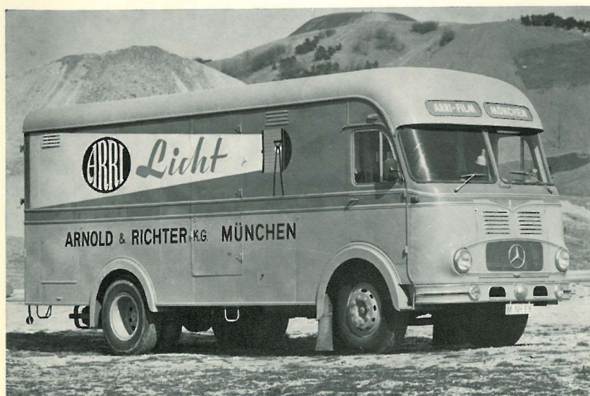
For large-scale lighting: Quiet-running three-phase aggregate 200 KVA 220 V/380 V with Mercedes diesel motor 250 HP in Mercedes van
