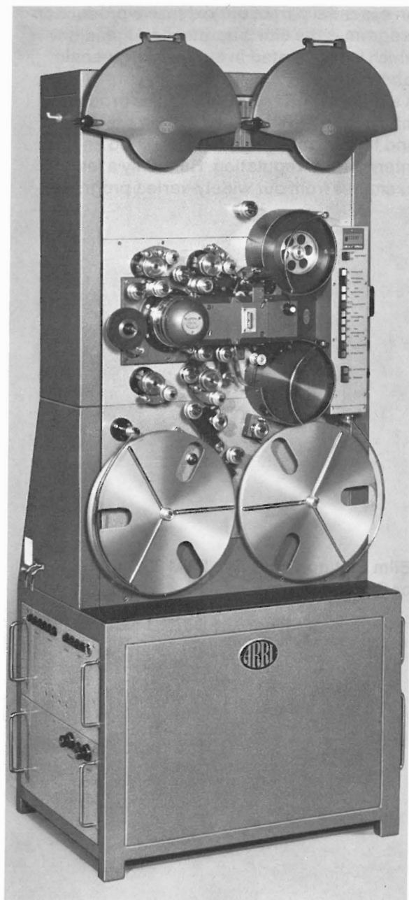
High Output Continuous Printing Machine Type DK/B, 16 or 35 mm, for B & W and color
