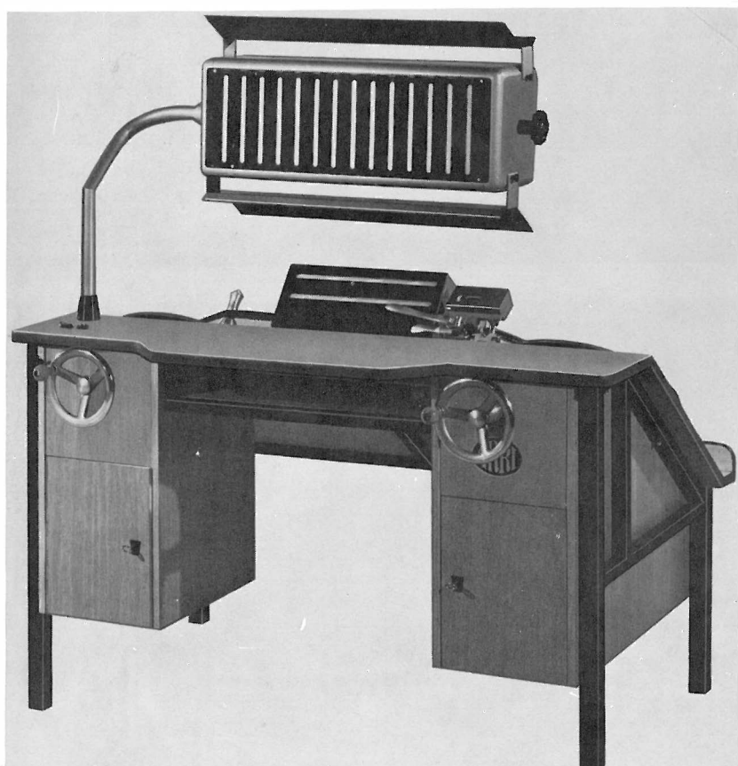
Color Analyser LT 16 for 16 mm film
